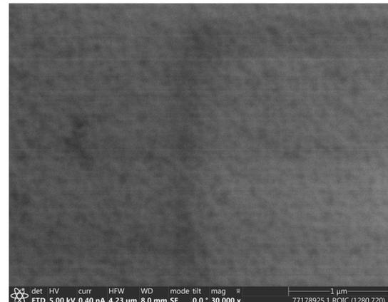
As can be seen in Figure 8, compressive stress in the AlN barrier film leads to a reduction in the “crystallite” formation in the AlScN films.
