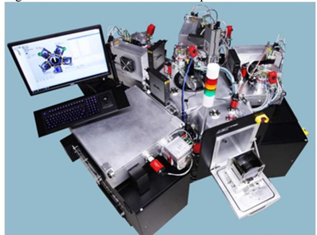
The trimming module uses DC focused ion source with up to 5kV acceleration voltage. This module was used for substrate surface clean up before deposition, as well as for improvement of surface roughness of the AlN barrier layer deposited before AlScN deposition.
