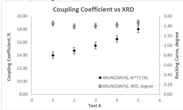
Since rocking curve doesn't always follow the coupling coefficient, see figure 4, and in order to investigate most important process parameters, simple HBAR devices were manufactured to measure  $kt^2$ .
